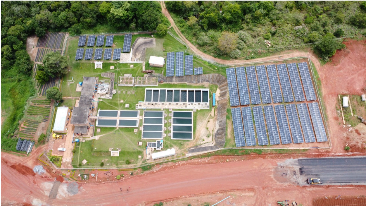
Hybrid Solar PV System with Solar Capacity 480.69kWp & BESS Capacity 1,295.77kWh at Mzuzu Treatment Plant
